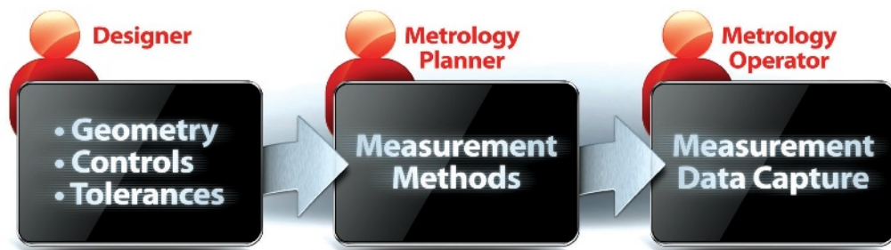
FIGURE 1: Three separate entities perform the what, how and when of part inspection. Image courtesy of InnovMetric Software.
