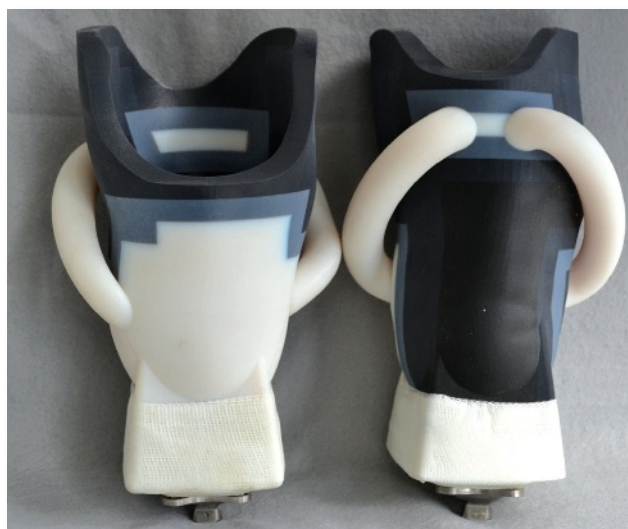
Sengeh used the Objet Connex 500 3D printer to create sockets that are customized for each patient based on an MRI scan. The printer’s ability to work with multiple materials with different stiffness and flexibility increases the socket’s comfort.
