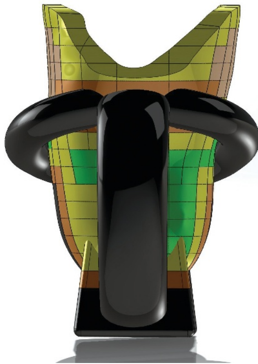
David Sengeh, a doctoral student at the MIT Media Lab, used SolidWorks and MathWorks MATLAB to design and virtually test the prosthetic sockets to improve their comfort for amputees.
